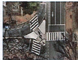
Aerial of intersection where a two-way street intersects with a three-lane one-way street. The intersection is signalized and has a pedestrian refuge island that connects the three crosswalks of each of the three road segments.
